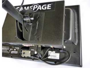
2. Connect the CAT5e running through the stand to the RJ-45 port on the bottom of the unit. Attach the provided coupler to the other end of the CAT5e on the stand.
